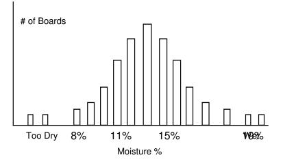
To determine the average MC - add up all the boards MC readings and divide this number by the number of boards measured.
